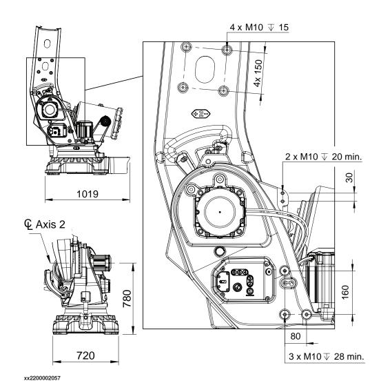
2.2 Fitting equipment on the robot (robot dimensions)
