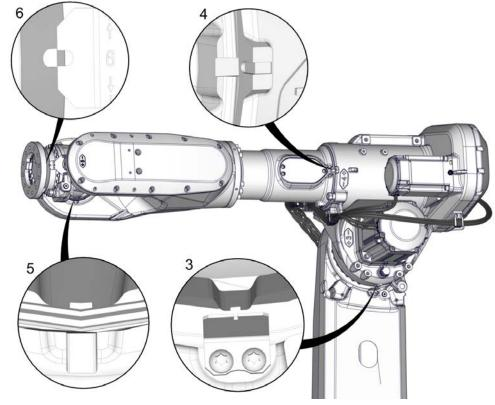
2.6.3 Calibration movement directions for all axes
